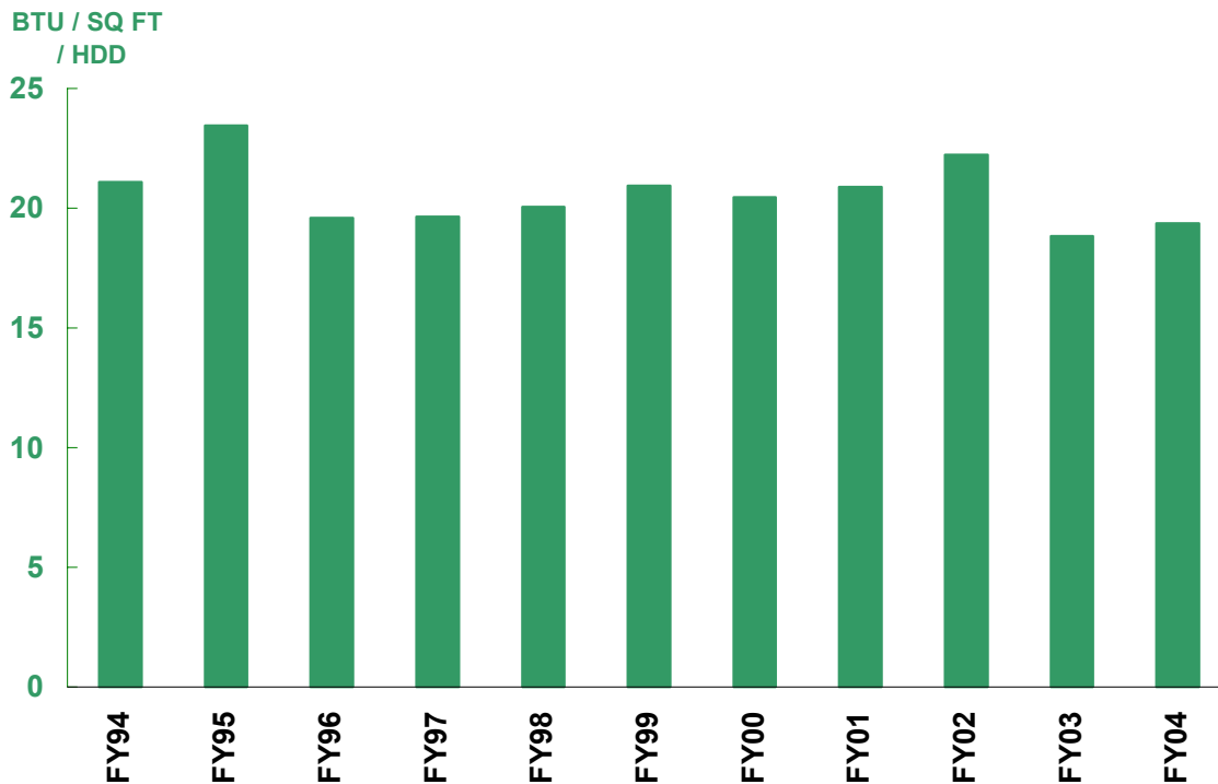
Figure A3 Main campus natural gas consumption normalized for winter weather in HDD and campus growth in square feet
