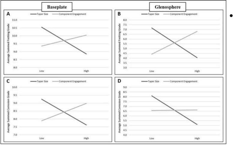
F&C grades on glenospheres with trunnions (component engagement; male; high) were significantly greater than glenospheres with bores (component engagement; female; low) (both p≤0.001)
