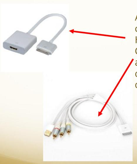
A TV can be connected with an HDMI adapter or a Composite Video adapter, depending on the type and age of the TV.
