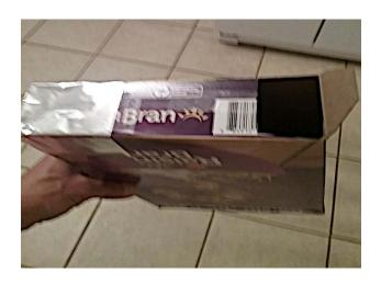
Now you have made a classic pin hole projection box. The sun will shine through this hole onto the white view paper screen on the other end of box. Use the small hole with flap to view inside. Remember to stand with the Sun, or eclipsed Sun, behind you as you look in the box.
